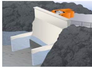
Fig.11 Fixed OWC-type WEC with side walls
