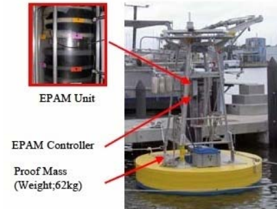
Fig.24 EPAM generator system on the test buoy
